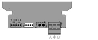
The inputs are provided on HD4 as shown, and are also labelled on the circuit board. Control inputs are for connection to voltage free contacts only. Internal pull-up resistor source current =  $33\mu$ A. These inputs form part of a TNV3 circuit and precautions must be taken to prevent hazardous voltages being applied to these circuits.
